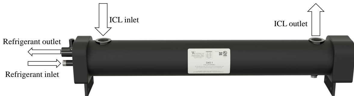
Fig. 2 The shell-and-tube heat exchanger and the ICL and refrigerant (R404-A) inlets and outlets
